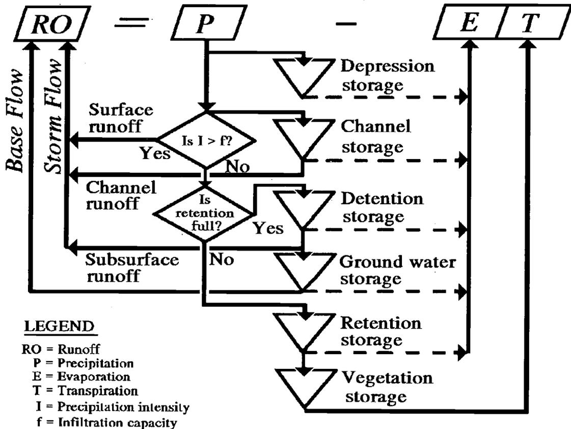
Figure 3. The Hydrologic Cycle Components Arranged by Storage Location and Function Within the Watershed.
