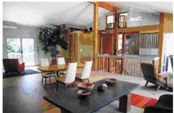
Fig. 13. The farmhouse interior with 100-year-old salvaged wood columns and engineered wood beams. The interior of the house is comprised of biobased, recycled, and reused materials as well as engineered lumber and low-to-no-toxin finishes. All furniture is salvaged, reclaimed, and renewed.
