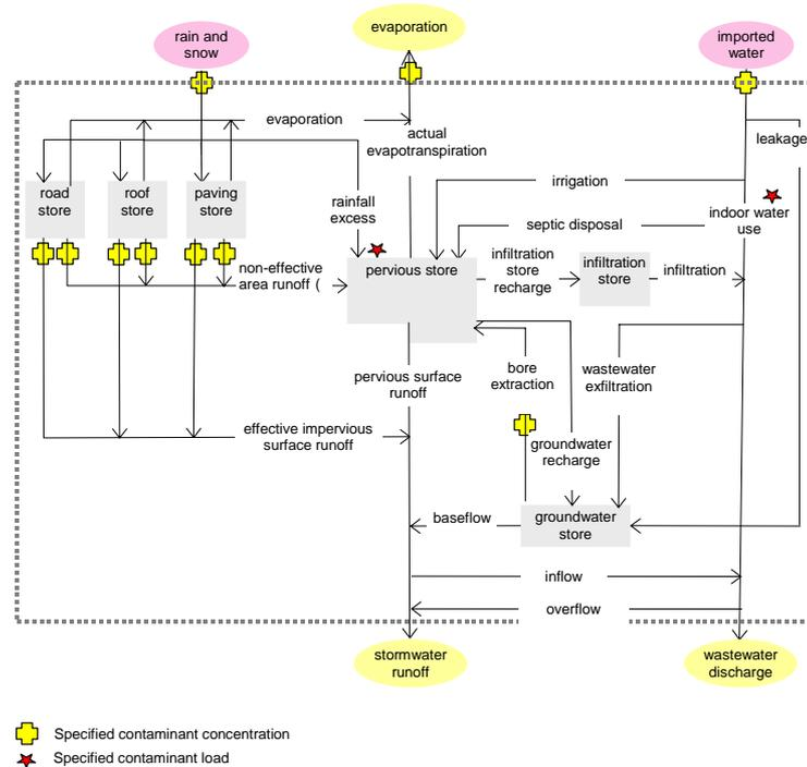
**Figure 1** UVQ representation of a conventional urban water system with separate sewers
