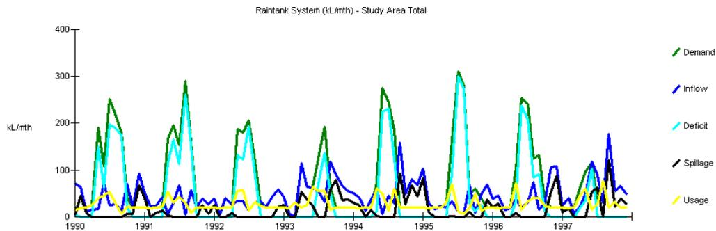
Figure 4 Example of rain tank behaviour output graph
