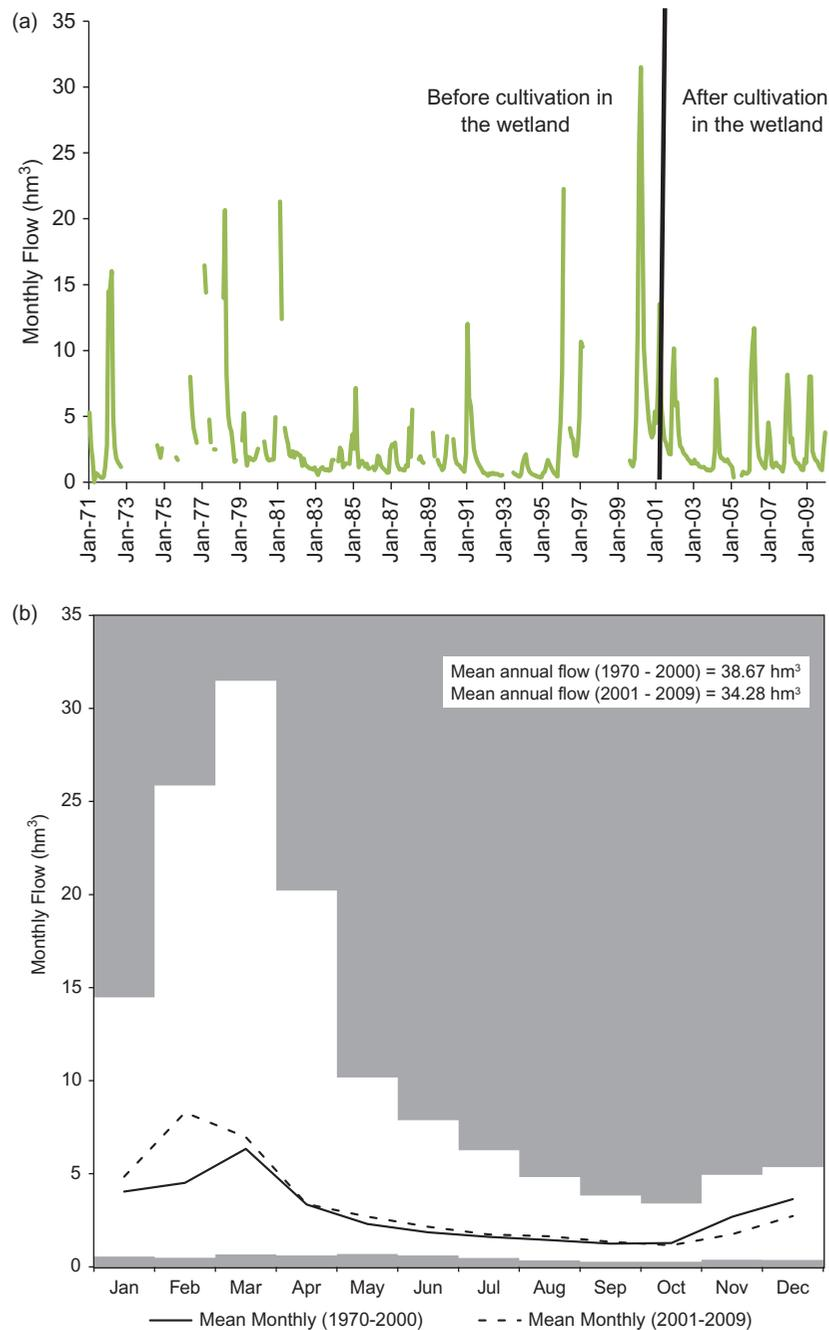
**Fig. 5** (a) Time series of Mohlapitsi flow measured at B7H013. (b) Comparison of mean monthly flow as measured at the B7H013 gauge for the periods 1970–2000 (dashed line) and 2001–2009 (solid line). The white bars indicate the monthly maximum and minimum flows measured between 1970 and 2000.
