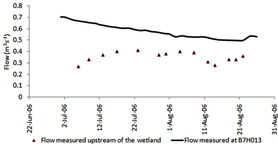
Fig. 7 Flow measured upstream and downstream of the wetland over the period 6 July–22 August 2006.
