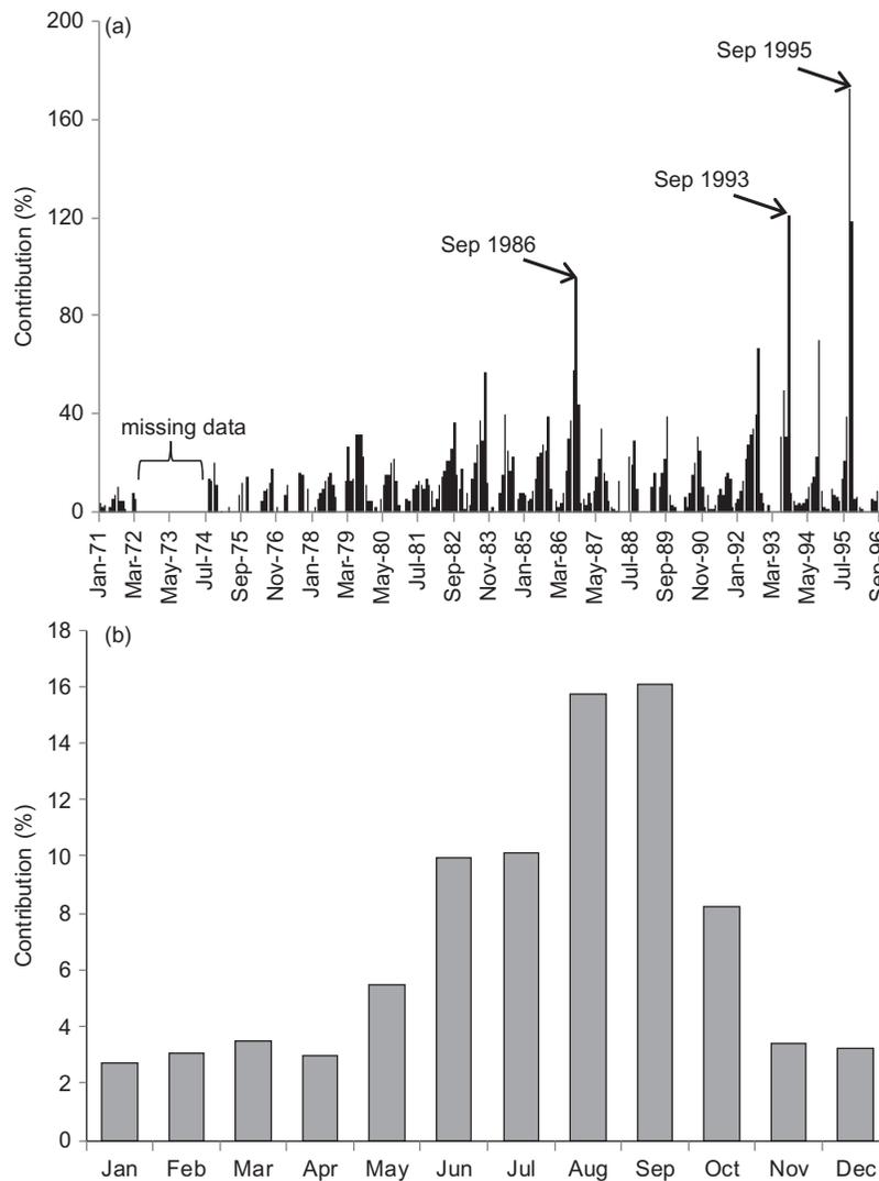
**Fig. 3** (a) Time series showing the percentage contribution of flow from the Mhlapitsi River (gauge B7H013) to the Olifants River (gauge B7H009). (b) Percentage contribution of flow (i.e. average monthly) from the Mhlapitsi River (B7H013) to the Olifants River (gauge B7H009).
