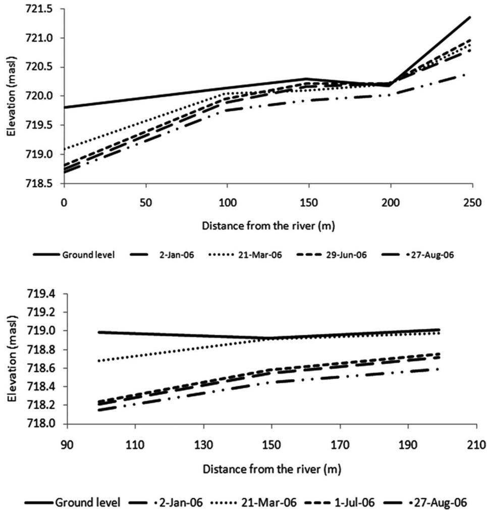
Fig. 6 Water table elevation on different dates along: (a) transect 1 and (b) transect 6.
