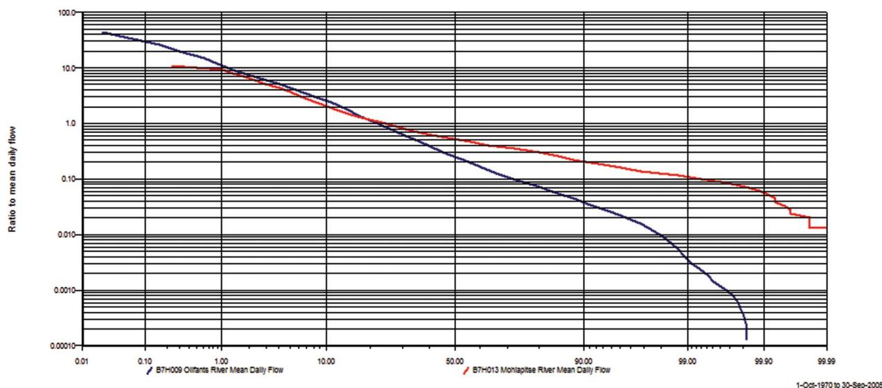
**Fig. 4** Flow duration curves (presented as ratio to mean daily) for both B7H013 (red line) and B7H009 (blue line).
